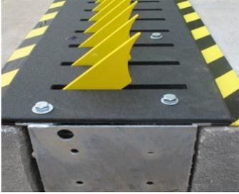
Install on a level surface whenever possible. The exact length of the LP72 model is 72 inches. Units are installed end to end and can be bolted together using the 4 holes at the end of the frames. Limit space between the units to .25 inches or less.
